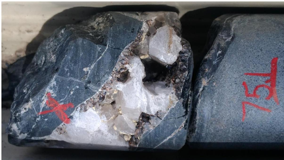
Photo: Quartz-Cassiterite vein at 75.1m in LDD003.
